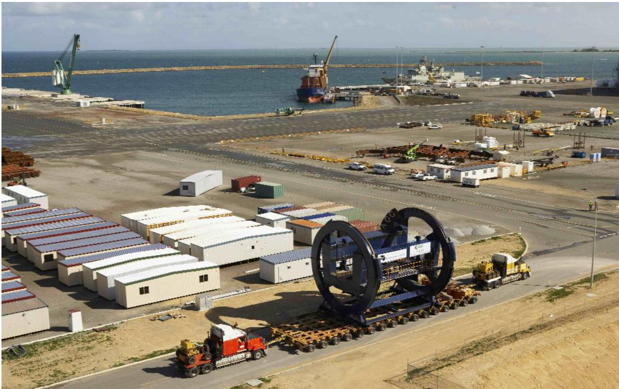
The first of the Tippler Cells being moved from AGC Kwinana to the wharf bound for Port Hedland.
