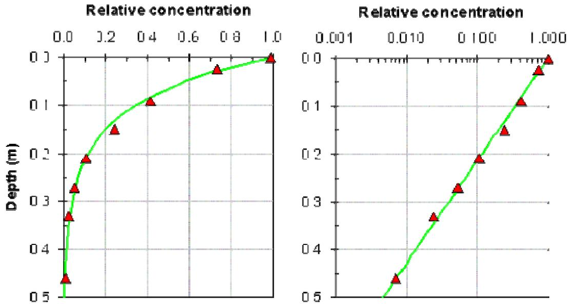
Figure 1. Relative oxygen concentration in a mine tailings column (after Yanful, 1991).
