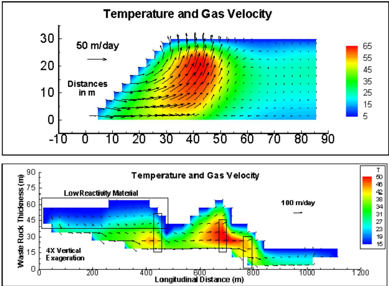
**Figure 6.** Simulated temperature and gas velocity for the Nordhalde (top, Lefebvre, Smolensky and Hockley, 1998), Doyon (center, Lefebvre, 1994) and Questa (bottom, Lefebvre et al, 2002) waste rock piles.
