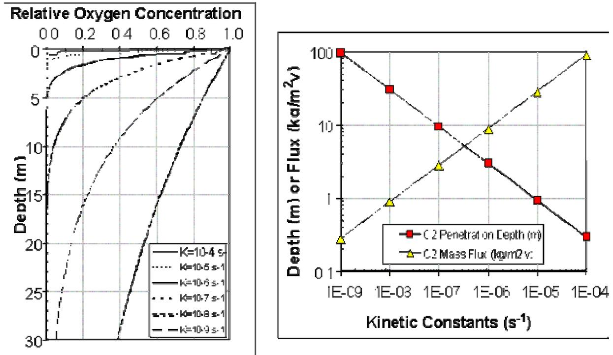
**Figure 2.** Oxygen diffusion as a function of the oxidation kinetics constant  $K$  ( $s^{-1}$ ). Left: oxygen profiles vs depth. Right: oxygen penetration depth at which the relative concentration is 0.05 and the related oxygen mass flux from the surface.
