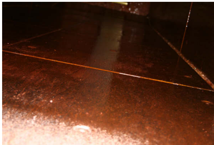
Figure 2. Surface of Skip treated with Alderox® ASA-12®
