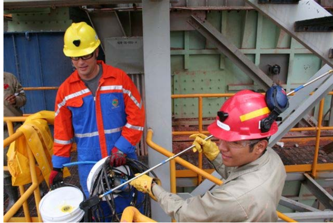
Figure 5. Peñoles miners with handheld bucket top sprayer system
