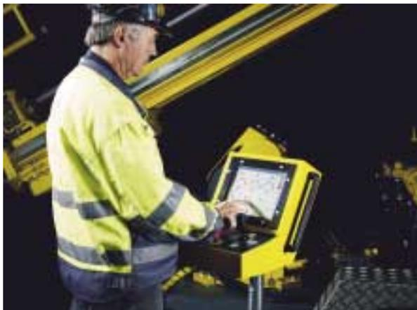
With the release of the fourth generation of its computerised control system APC, for the Diamec core drills, Atlas Copco has taken another step to increase productivity. By using the APC with the Diamec rig, the cost of consumables can be lowered significantly in any surface or underground core drilling. The APC makes it easier to control and maintain a more efficient drilling, which prolongs service life of diamond bits and ITH tools
