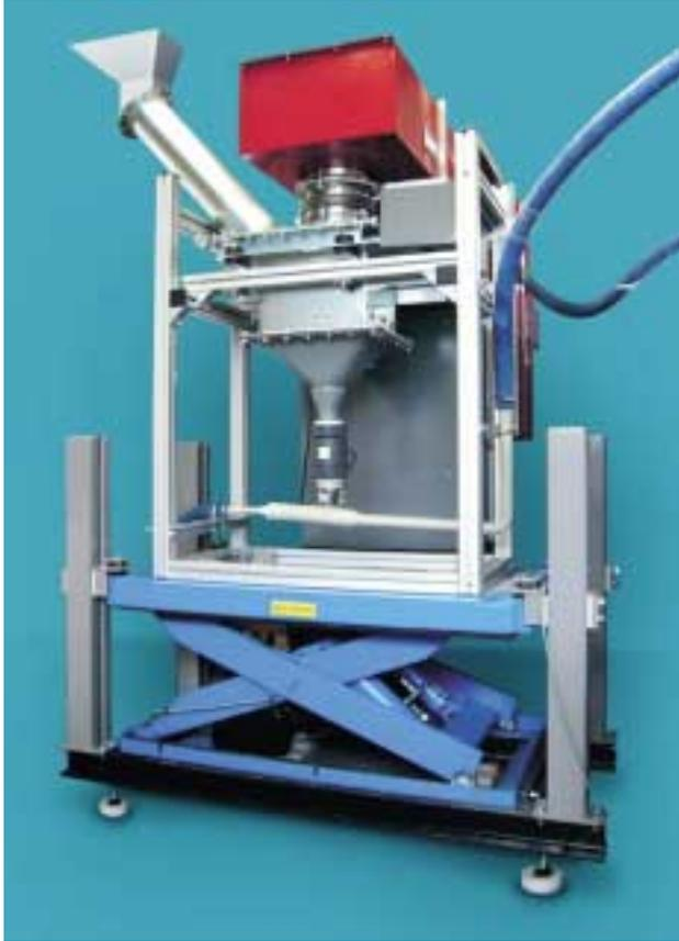
*selfFrag provides what it claims is the first commercially available continuously operating HV-pulsed power device to process exploration mini bulk and batch samples for further analysis*
