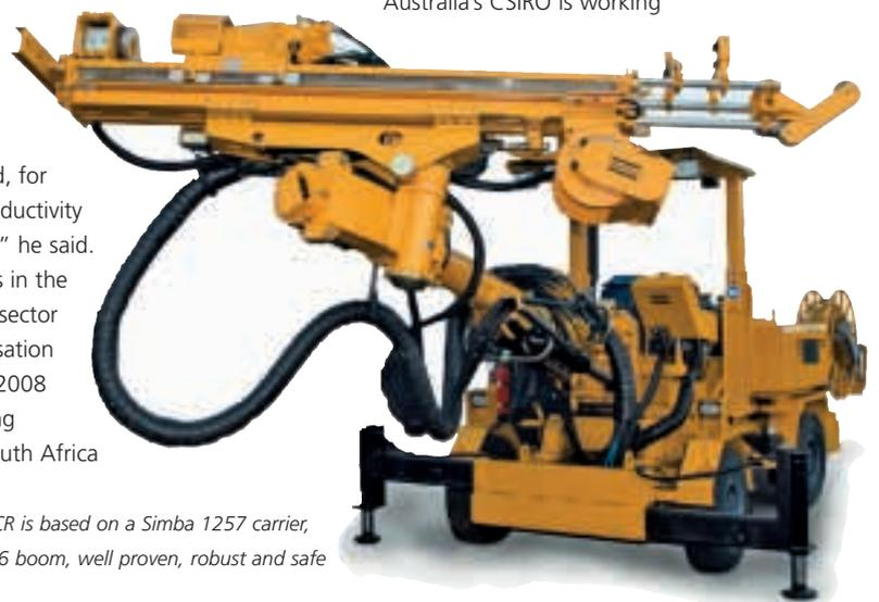
*The Diamec MCR is based on a Simba 1257 carrier, and a Diamec U6 boom, well proven, robust and safe components*
