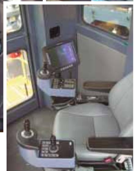
RCS basic replaces electric joysticks (top right) in the latest Atlas Copco Pit Vipers, PV-271/5 (above) and PV-351 (right)
