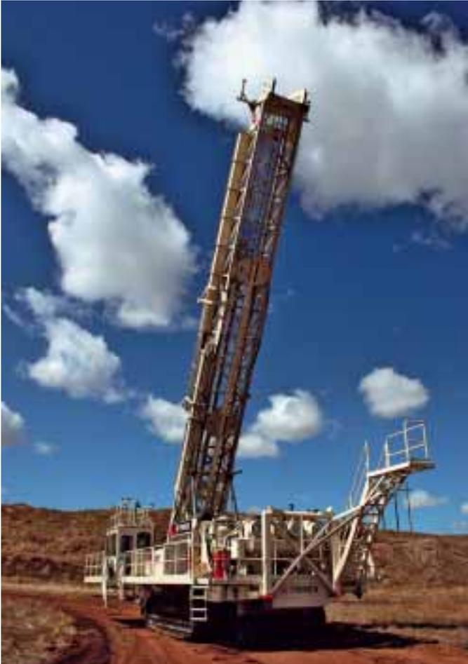
All Terex rotary blasthole drills, including the SK-L, are manufactured with the patented Hydraulically Operated Break Out wrench (HOBOW), designed to increase drill productivity. It allows for a method of breaking joints that is both simple and safe for the operator
