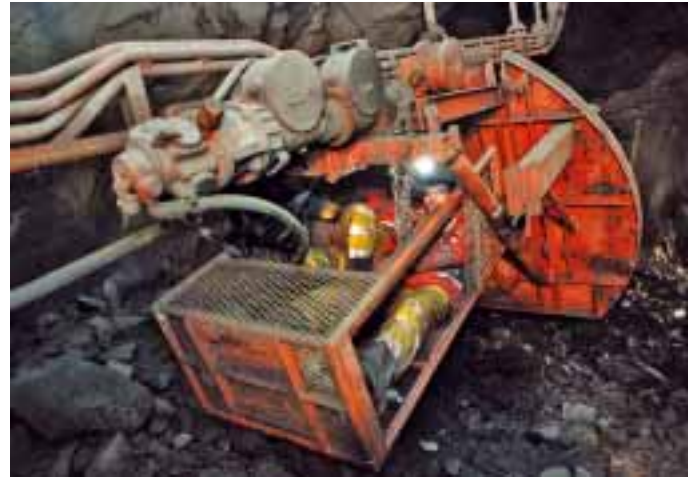
Alimak raise miner in action. Picture by Eija Hiltunen
