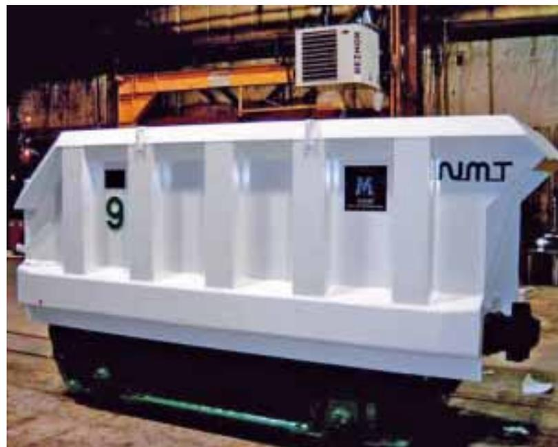
A Nordic Mine Technology 5 m<sup>3</sup> end hinge mine ore car
