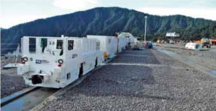
*Mining Equipment Ltd 25 t diesel locomotive pulling 15 m<sup>3</sup> capacity roll-over muck cars through a dump at OK Tedi mine, Papua New Guinea*
