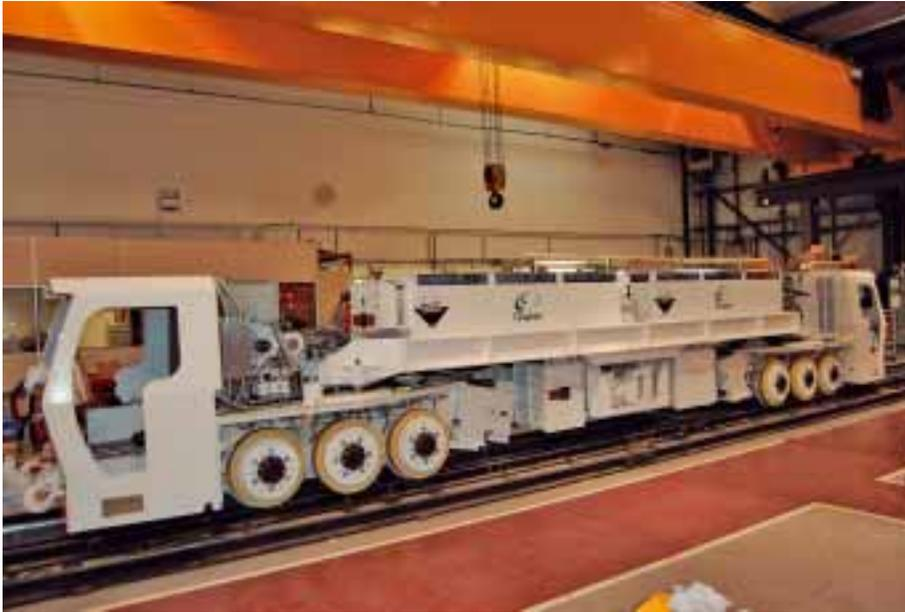
*A Clayton 30 t rubber tyred flameproof loco during tests in its UK factory*
