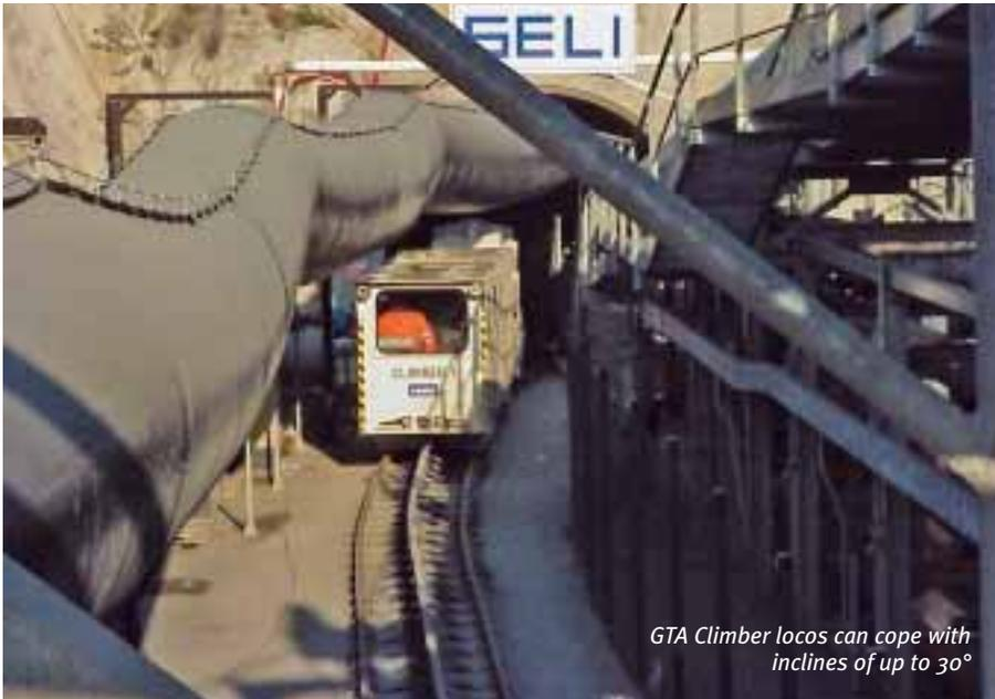
*GTA Climber locos can cope with inclines of up to 30°*
