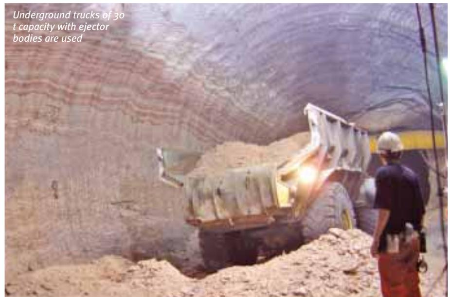
*Underground trucks of 30 t capacity with ejector bodies are used*
