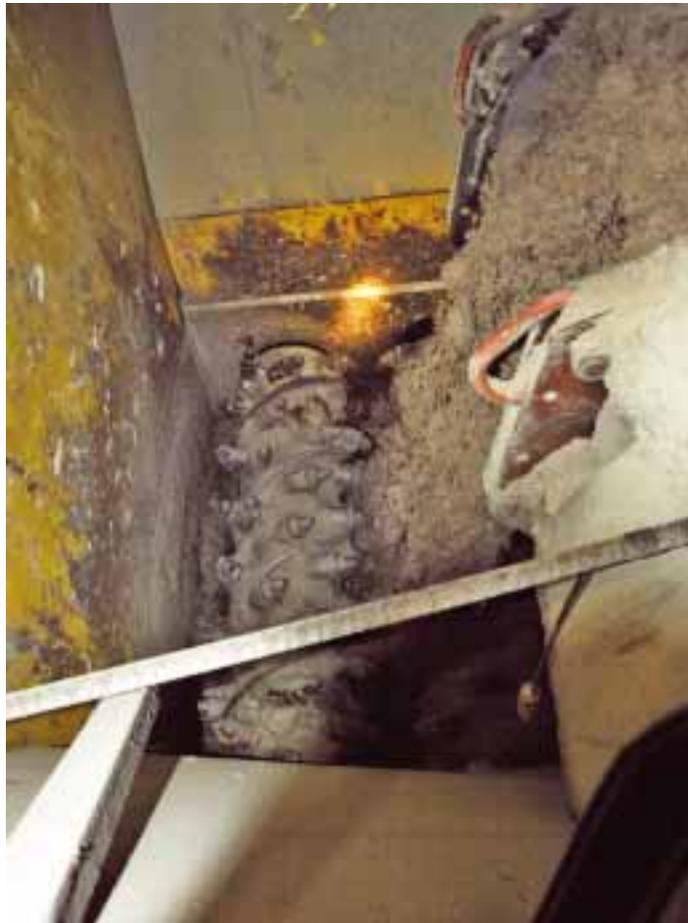
*Sylvinite ore entering feeder breaker before being conveyed to the hoist level*
