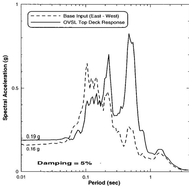
Fig. 8. Base input and OVSL landfill top deck response to Nisqually earthquake in east-west direction
