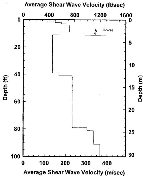
Fig. 7. Average shear wave velocity profile of OVSL site
