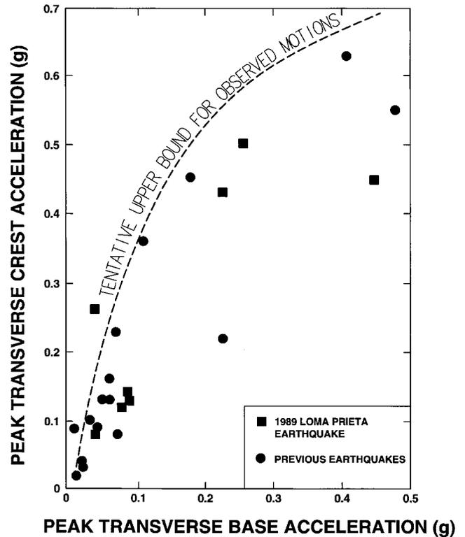
Fig. 6. Approximate relationship between peak base acceleration and peak crest acceleration at the crests of earthen dams [transverse direction] by Harder (1991), with permission
