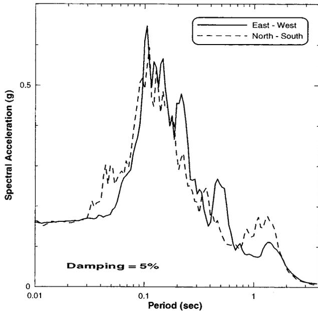
**Fig. 3.** Strong-motion records recorded in soft rock approximately 1 km from the OVSL site
