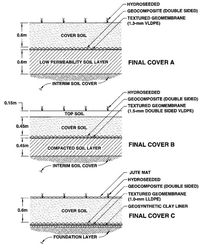
**Fig. 2.** Composite cover configurations of the OVSL site [data adapted from GeoSyntec Consultants (2003)]
