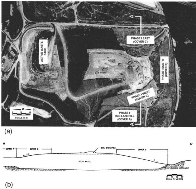
**Fig. 1.** (a) Aerial photo of the landfill six months after the February 28, 2001  $M_w$  6.8 Nisqually, Washington earthquake, and (b) cross section A-A'
