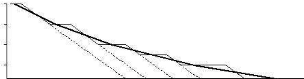
Figure 22: Stepped profile to achieve concave profile with minimum dozing
