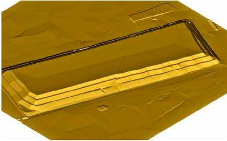
Figure 5: Typical Heap leach pad
