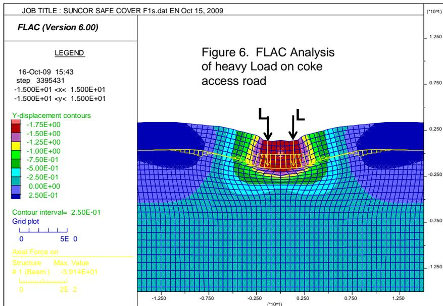
Detail of 'F1s' file (Coke thickness = 3m & geogrid stiffness = 350 kN/m) with vertical displacement contours in meters. (L = 110 kN/m & max tension in grid = 39.1kN/m)
