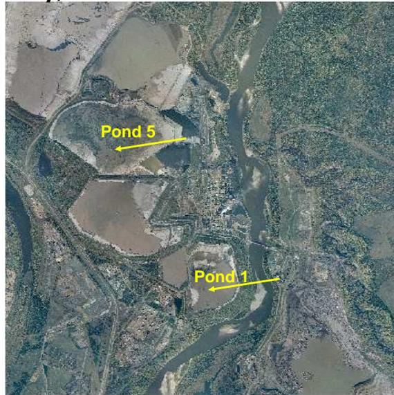
The tailings vary considerably. The upper layer is very soft, low strengths (less than 1 kPa) clayey materials that are still essentially fluid at void ratios of up to five. The strength and sand content increase with depth to the bottom of the pond that is deeper than 50 m. (Figures 2 and 3.)
