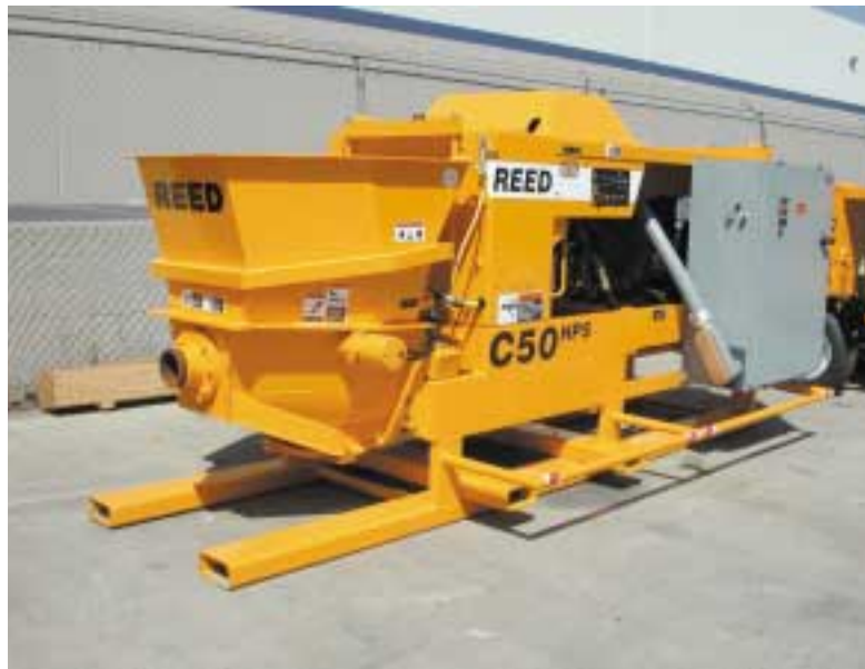
REED Manufacturing's new 'Mine Version' C50HPS-SKE shotcrete pump was specifically designed for extremely long distance underground applications. Powered by the combination of a 93 kW electric motor and 180 cc main hydraulic pump, it has a maximum output of 40 m 3 /h, 129 bar concrete pressure. The very high performance of this shotcrete pump is required on many jobs where shotcrete needs to be pumped hundreds of meters before it is sprayed.
