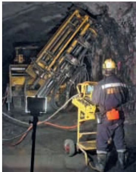
Drilling a production ring blast pattern with a Simba H-254
