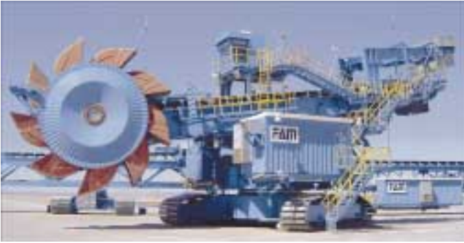
FAM bucketwheel reclaimer – compact design, capacity 4,000 t/h of ripsos
