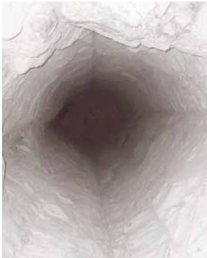
Hole drilled for inverse drop raising
