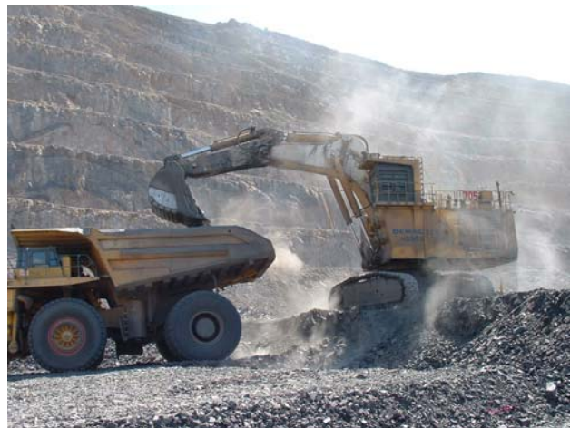
Photo 1 Excavator at Century Zinc Mine equipped with GPS guidance for selective mining of ore.
