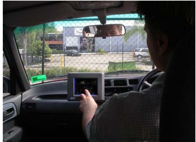
Photo 5 Foreman's vehicle system equipped with wireless LAN to duplicate Shovel operators view.
