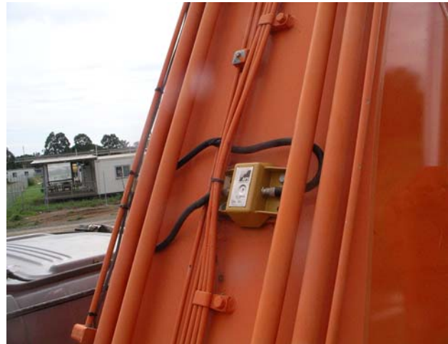
Photo 6 Tilt Sensor Installed on excavator boom.
