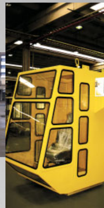
Cabine de ponte rolante Cabin of crane
