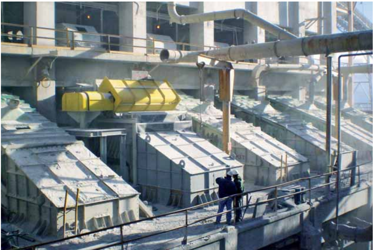
Screening machine with direct exciter drive for processing copper ores
