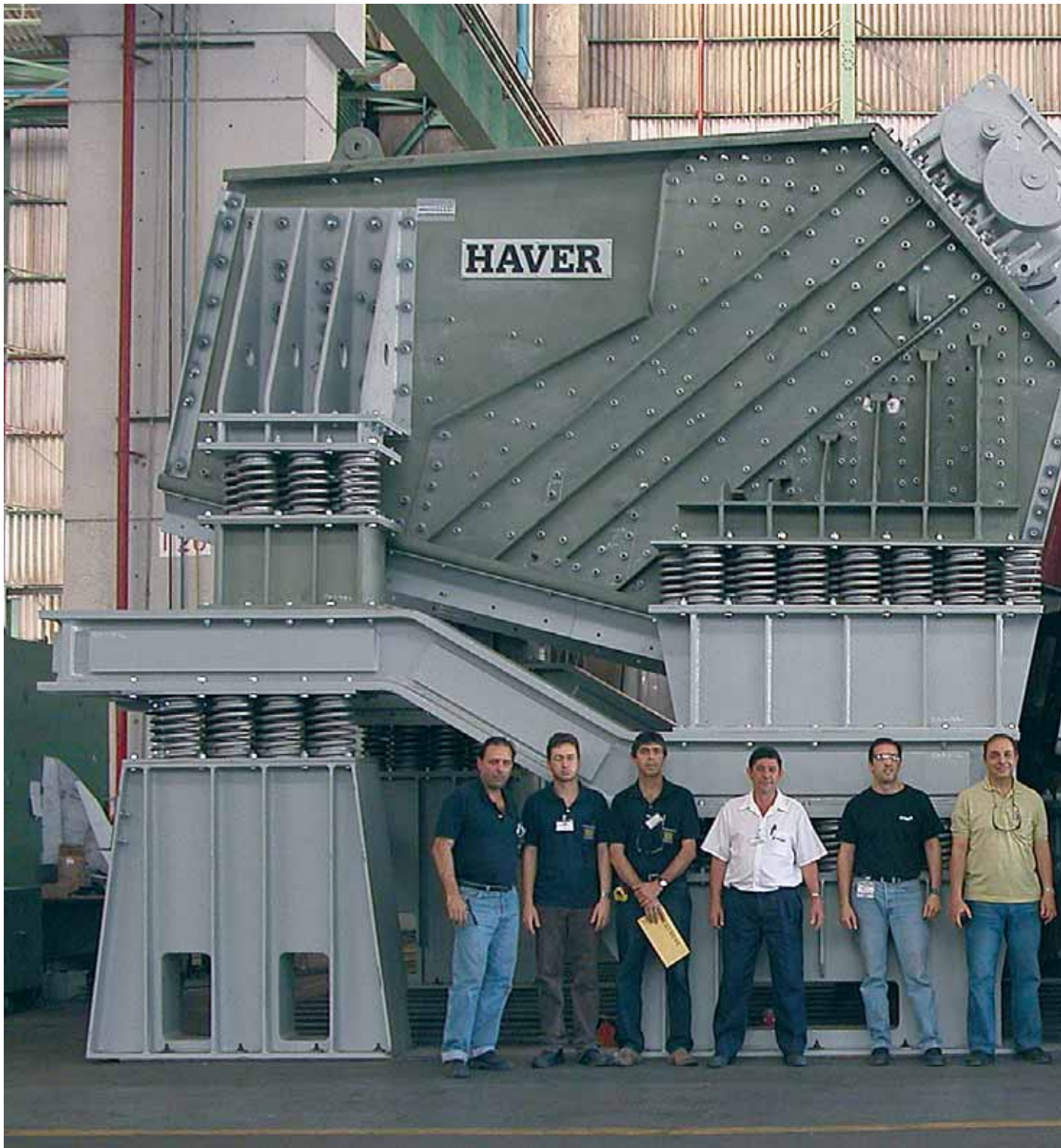
NIAGARA® High performance screening machines in modular design, Type R-TE 4000 x
