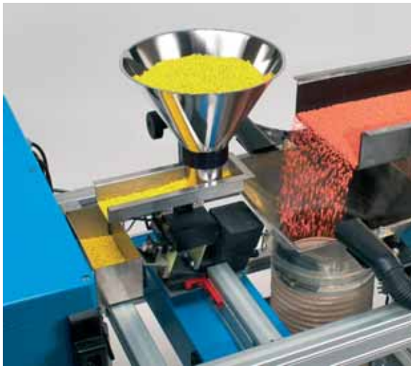
The HAVER CPA photo-optic particle analysis unit for performing particle size and shape analyses
