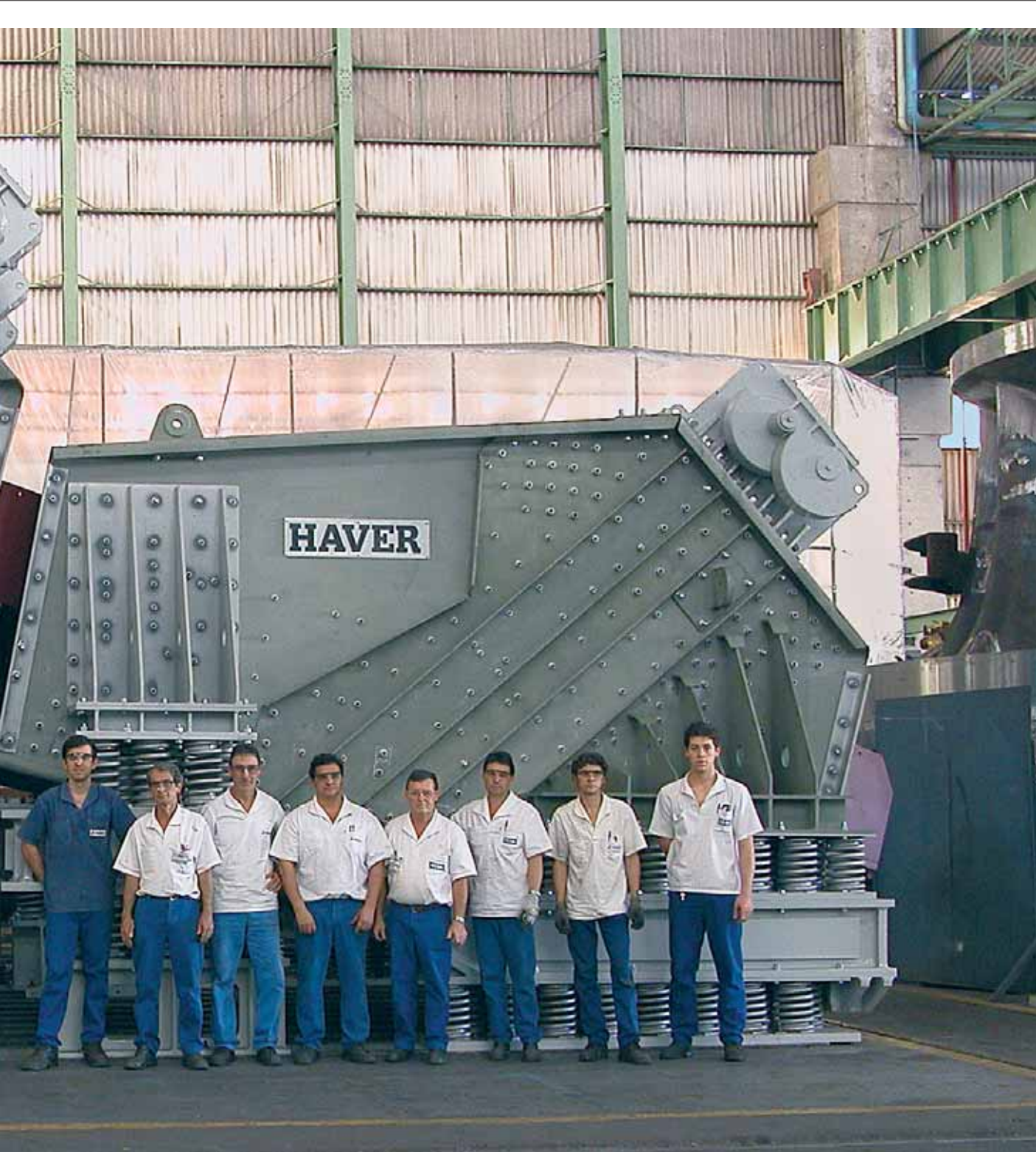
11000, total weight of 115 tons, 15000 tons of oil sand per hour
