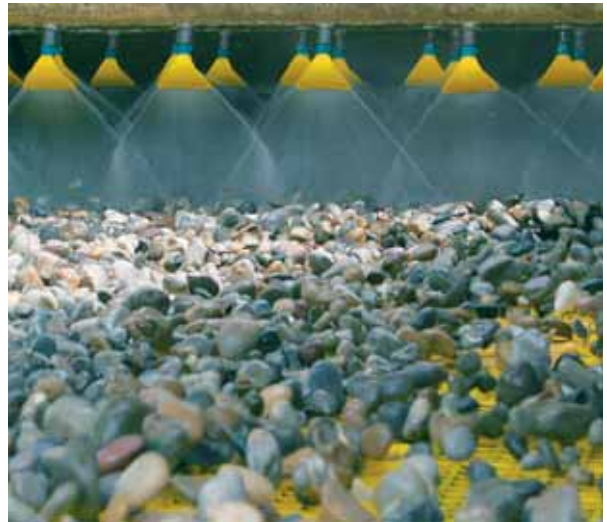
HAVER NIAGARA® flat screen with spray bars FL-MD 2000 x 6000, round gravel, 200 tons/hr
