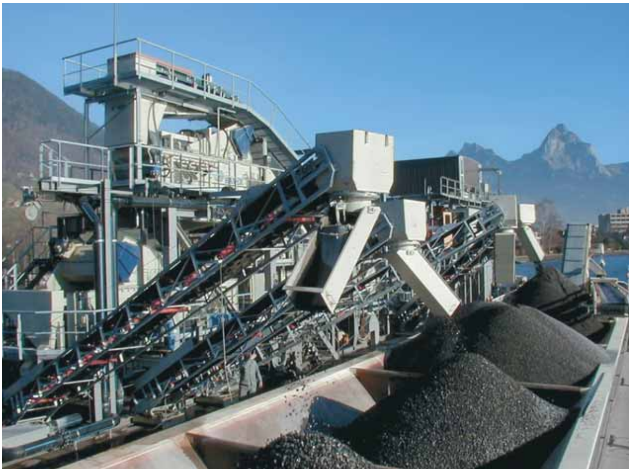
Dredging ship equipped with HAVER NIAGARA® flat and de-watering screening machines and HAVER vibrating feeders, gravel, 200 tons/hr
