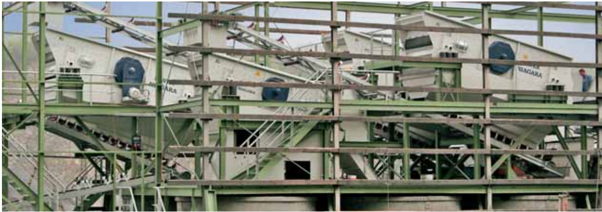
NIAGARA® Free-Line, 3 x MD 1800 x 5000, 1 MD 1500 x 4000, culm basin carbonate, 220 tons/hr
