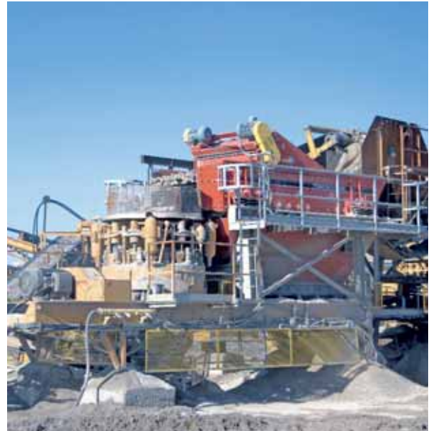
Screening machine with double-shaft drive system for the gravel industry
