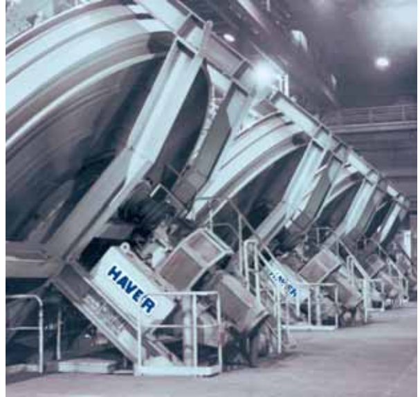
Giant pelletising plates Model GR 7500, 122.3 tons/hr
