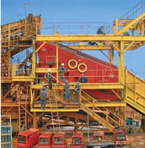
Free swinging scalper with double-shaft drive system for processing nickel ores
