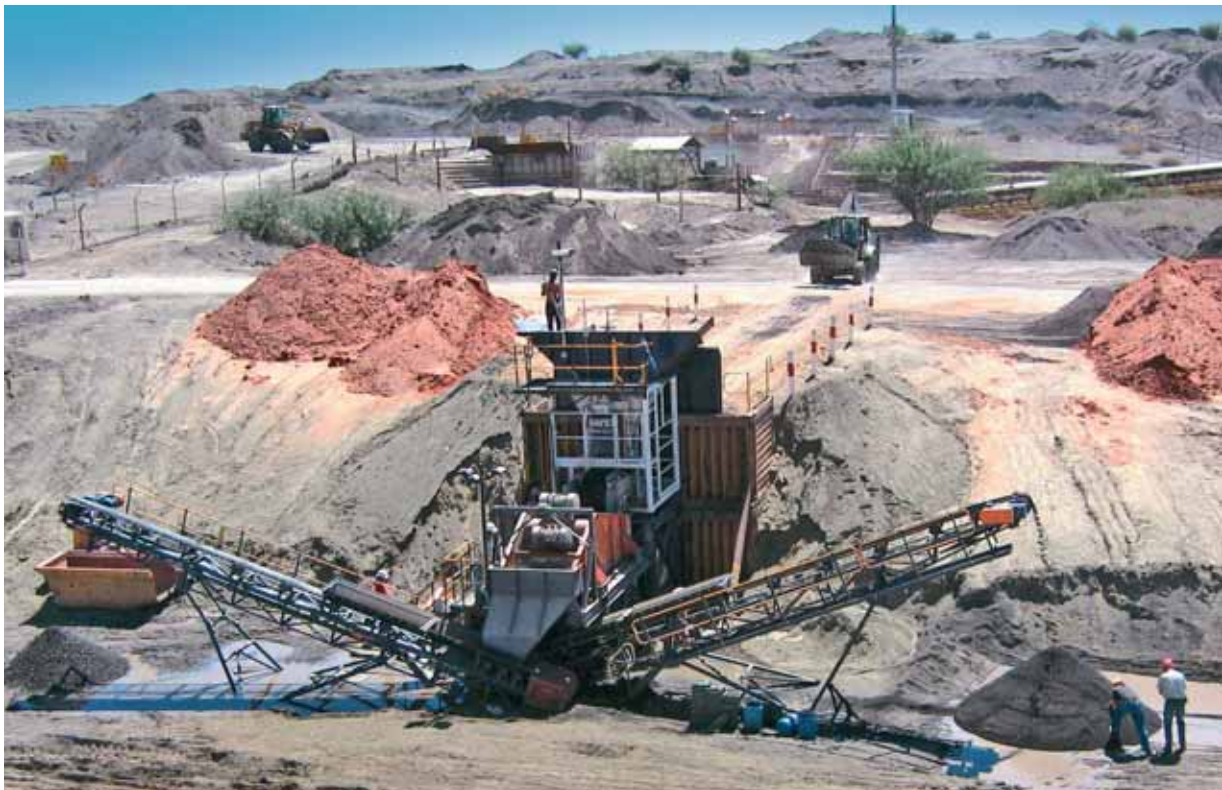
Semi mobile HAYER Hydro-Clean® pilot plant, HC 700/200, for kimberlite, 50 tons/hr
